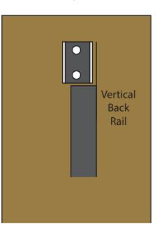
**B** Attach one vertical back rail to each post, using (5) 5/8" screws.
