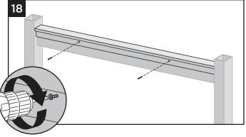
**18.** Install (1) #10 x 2" self-drilling pan head screw into each predrilled hole. Tighten the screws until the picket is clamped in the top rail such that it cannot move up or down.
