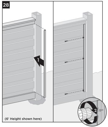
**28.** Replace each L-channel in same location as in steps 25/26, and attach to the post using (1) #8 x 1" pan head screw at each predrilled location.
