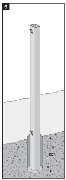
6. Set the posts at the desired spacing with an embedment of 30". Ensure posts are plumb and level. Fill holes with code approved concrete and allow this to fully set before attaching fence components.
