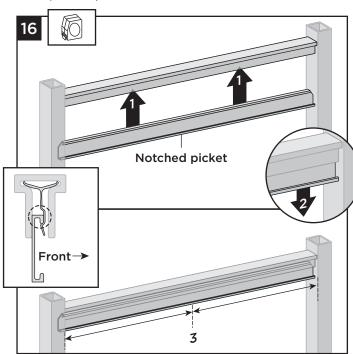
16. Install the first picket (with the notched side up) into the top rail with the open side of the picket facing the FRONT of the fence assembly. Push the picket up (tapping gently with a rubber mallet if needed) so it fully engages with the snap feature on the aluminum insert. Once fully engaged, pull down on the picket so it seats properly in the top rail. Ensure the picket is centered between the posts.
