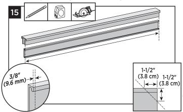
**15.** Cut the first picket 3/8" shorter than the top rail. In addition, notch both ends of the first picket at  $1-1/2" \times 1-1/2" \times 45°$ .
