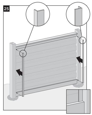
**25.** Position each L-channel against the post with the short leg against the post and the long leg extending over the pickets. Insert the short leg between the post and the ends of the pickets so the long leg is flush against the pickets and aligned with the inside edge of the top and bottom rails.
