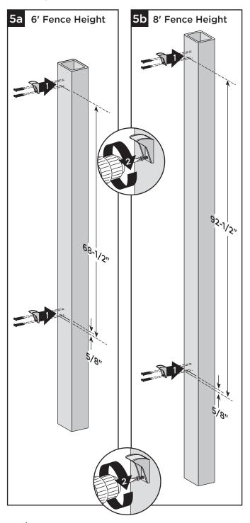
**5a/5b.** Install the top and bottom brackets on the posts using (4) #8 x 1-5/8" flat head screws per bracket.
