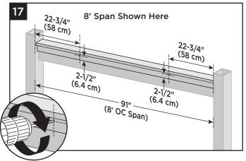
17. On the BACK of the fence assembly, predrill thru the aluminum insert using a 1/8" drill bit at the quarter points of the top rail approximately 2-1/2" from the bottom edge of the rail. Adjust quarterpoint measurements accordingly for smaller post spans.
