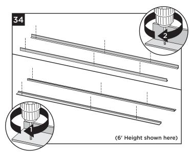
**34.** Remove each L-channel, and predrill holes at the locations marked in steps 32 and 33 using a 1/8" drill bit. **DO NOT** predrill posts or pickets.
