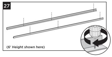
27. Remove each L-channel, and predrill holes at the locations marked in step 26 using a 1/8" drill bit. DO NOT predrill the posts.
