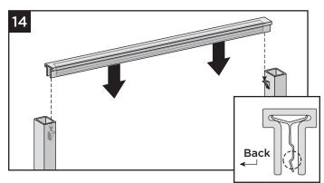
**14.** Set the top rail onto the top brackets such that the hook feature on the aluminum insert is pointing toward the **BACK** of the fence assembly.
