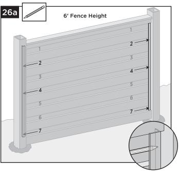
**26a.** Marking L-channels for attachment to posts on FRONT side for 6' fence height: Mark (3) locations on each L-channel, starting from the top, mark the 2nd, 4th and 7th openings in the infill where the L-channel's short leg is visible.
