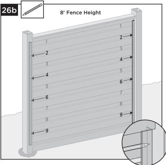
**26b.** Marking L-channels for attachment to posts on FRONT side for 8' fence height: Mark (4) locations on each L-channel, starting from the top, in the 2nd, 4th, 6th and 9th openings in the infill where the L-channel's short leg is visible.
