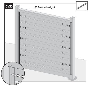
**32b.** Marking L-channels for attachment to posts on BACK side for 8' fence height: Mark (4) locations on each L-channel, starting from the top, mark the 1st, 3rd, 5th and 8th openings in the infill where the L-channel's short leg is visible.
