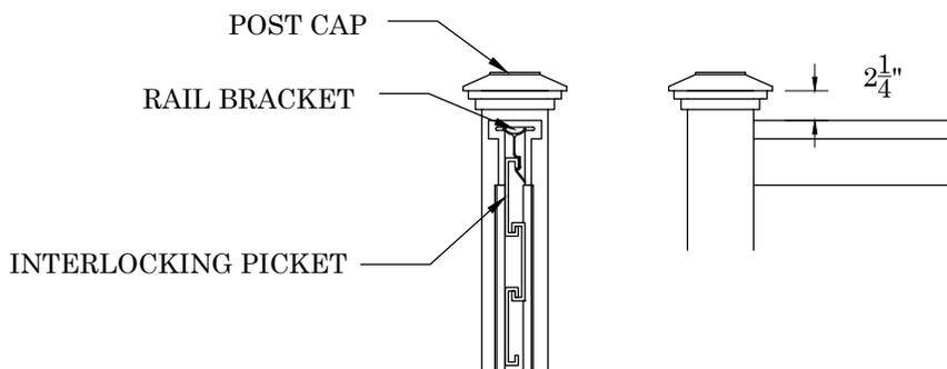
POST PROFILE: CUT VIEW/ELEVATION VIEW
